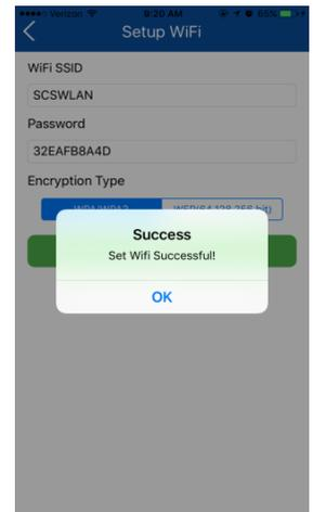
**Step 9:** Return to your controller and press the SET UP button one more time. Your controller’s LEDs will begin flashing in what appears to be a random sequence, indicating your controller is now paired to your router and is attempting to connect to the internet. Once internet connection has been established, LED1 will remain flashing and LED2 will be solid. This process normally take 2 to 3 minutes.
