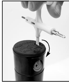
**DECREASING THE ARC:** Make sure the nozzle turret is in the right start position and insert the flat end of the plastic key on the universal tool into the arc set adjustment slot. Then turn the universal tool counter-clockwise. Each full 360° turn of the universal tool will decrease the arc 90°. Adjust to any arc between 40° and 360°. When you reach the 40° arc, the universal tool will stop turning or you will hear a ratcheting noise.
